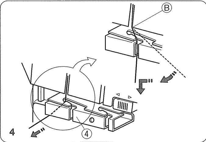
4. Hook the thread on the corner **B**, and then pass the thread through the looper thread guide.
