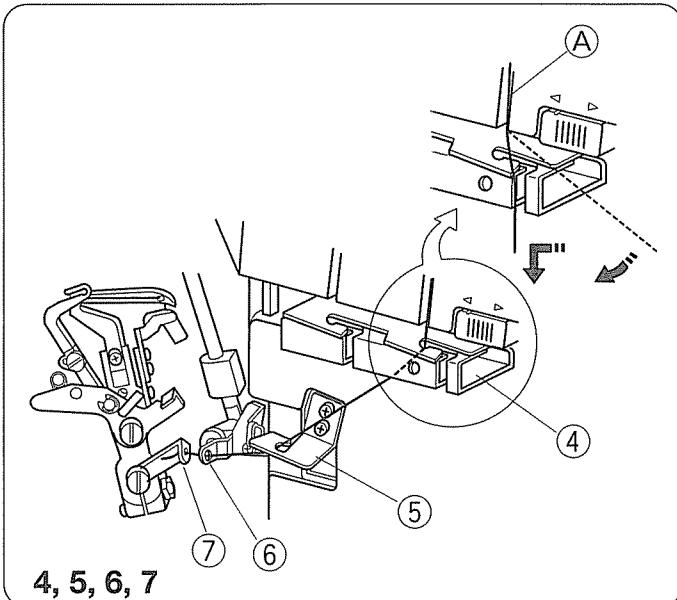
4. Hook the thread on the corner **(A)**, and then pass the thread through the looper thread guide.
