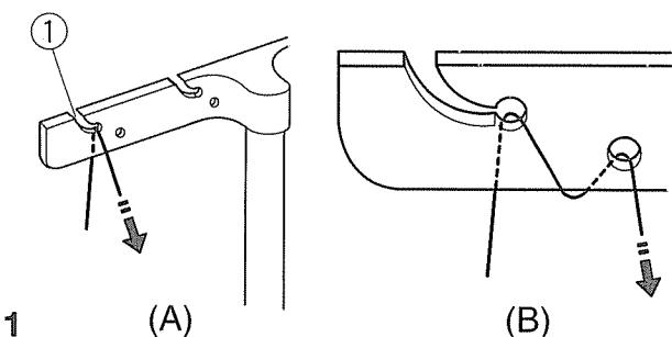
1. Draw the thread through the thread guide on the left from back to front: A
