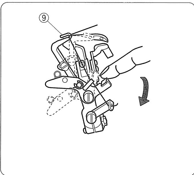
Holding the end of the thread, push the lower looper thread guide (1) down with your other hand to return it to its original position.
