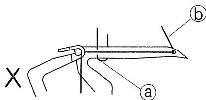
10. Move the lower looper to its rightmost position by turning the handwheel, and draw the thread with a pair of tweezers through the hole on the lower looper 10 cm (4') or more.
