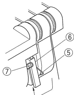
4, 5, 6. After passing through the front cover thread guide (1), pass the thread from the bottom of the front cover thread guide (2) and the take-up lever cover from right to left.
