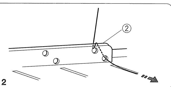
3. Hold the thread at both ends and tug gently to ensure the thread is correctly inserted between the tension discs. (If the presser foot lifter is raised, the thread easily inserts between the tension discs.)
